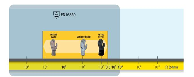
According to EN16350, electrostatic properties of protective gloves, the electrical resistance through a glove must be less than 10<sup>8</sup> Q. These gloves help protect you from the risk of explosion by dissipating (as much as possible) the electro-static electricity naturally present in the human body. They must be used in conjunction with shoes and antistatic clothing. The user must also be grounded. The performance obtained on our gloves ensures a high level of efficiency.
