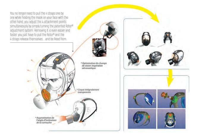
One of the key points to evaluate the performance of a complete respirator, and therefore the protection optimised for the user, is the adjustment. A good mask is in fact useless if the user adjusts it incorrectly on his face. Moreover, in some work situations, you have to work quickly and well. From this observation was born our idea to develop a complete mask that can adjust ultra quickly.
