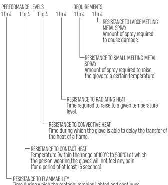
Time during which the material remains lighted and continues to be consumed after the ignition source has been eliminated.
