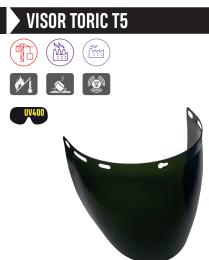
Marking (EN166) 1 = the best optical class A = the highest impact resistance T = impact resistance at extreme temperatures 9 = resistance to the projection of molten metals
