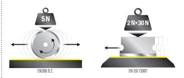
**ANSI ISEA (US American National Standards Institute) 105** Classification and specifications for the protection of the hand. Part 5.1.1. Cut resistance Weight necessary for a straight blade to cut the sample in a single movement.
