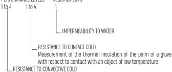
Measurement of the thermal insulation of a glove with respect to an ambient atmosphere.
