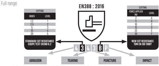
For gloves made of very resistant materials (materials that blunt the blade during the test), the Coupe Test is no longer relevant, a TDM test becomes mandatory. The TDM test is also more representative of work situations with high risk of cut.
